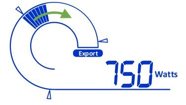
When the gauge moves in the direction of green arrow and the export symbol is shown, your household is generating more power than it is using and therefore exporting some power onto the grid. The value of energy available to use is shown in Watts. The Solar iBoost+ will be diverting energy to your immersion heater unless the tank is hot.
